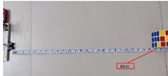
Fig 6.2 – Distance between the sensor and the object
