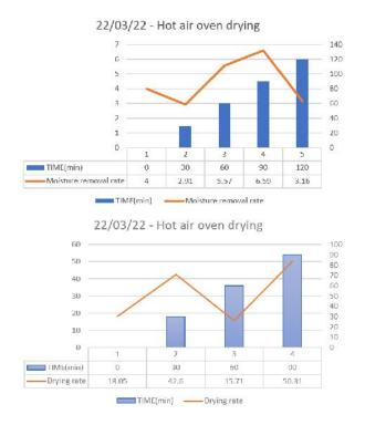
This line graph depicts that for moisture removal rate is has fall in first step after that it has increase drastically and decrease, comparatively in drying rate is fluctuated. This method is done in hot-air oven but it has not much give as expected result.
