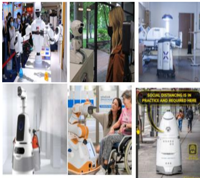
Fig. 31 Robots for COVID-19 diagnosis, Robots for screening, social and care robots. Security robots, sanitizing the hospital robots etc. [30].
