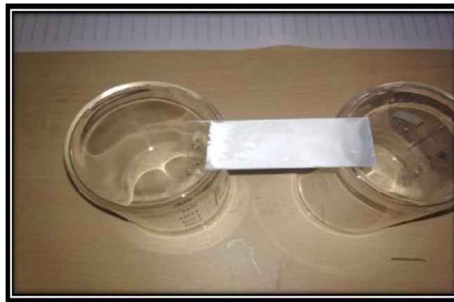
Fig-5 Developed PbSe thin film by CBD method.
