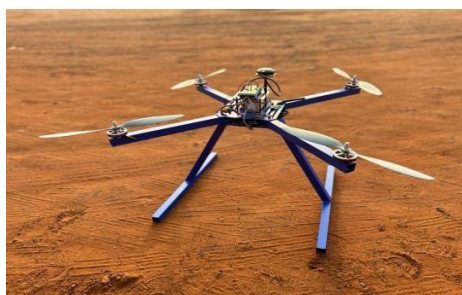
Fig 13 Autonomous organ transportation drone
