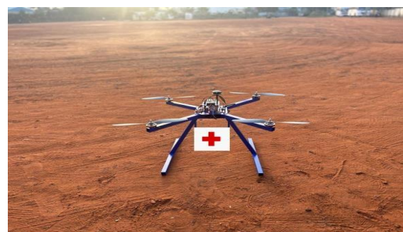
Fig 13 Autonomous organ transportation drone
