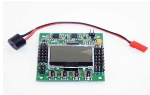
Fig 8 flight controller board
