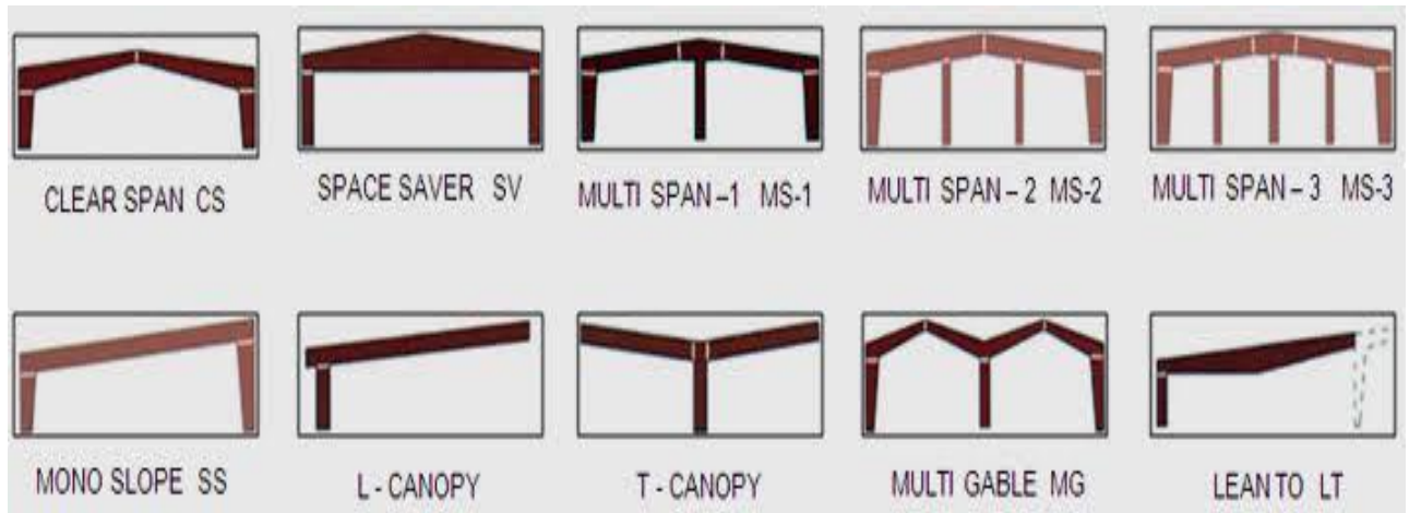
Figure: 03 - Primary framing structure.
