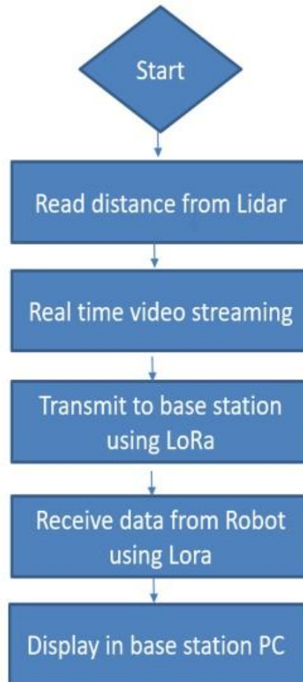
Figure 3. Flowchart from Bot to Base station
