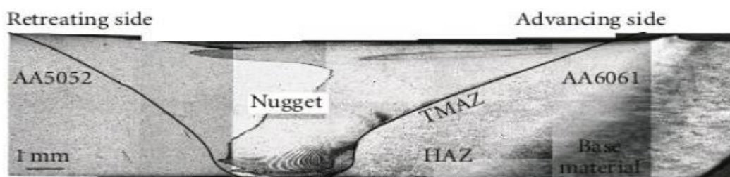
Fig 3. Motif of optical images of the transverse cross-section of FSW AA5052-AA6061 R1400F080 specimen showing the various regions [24]
