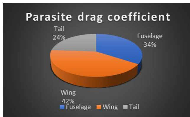
Fig. 15. Parasite drag coefficient contribution
