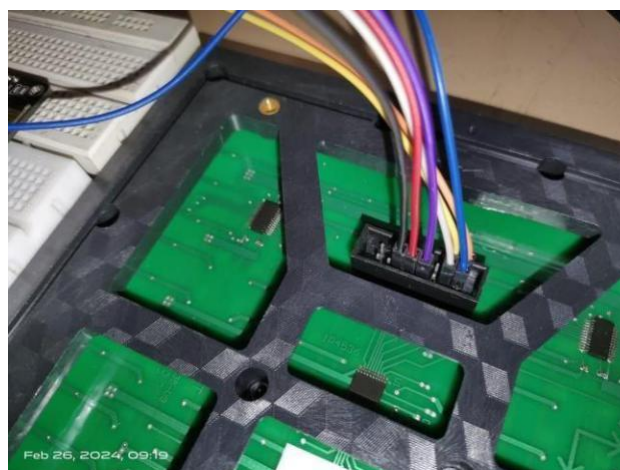
Fig. 5. Connections made to the p10 Matrix Display
