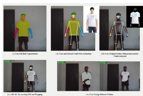
Fig. 8. AR pipeline: MediaPipe → SegFormer → TPS → 2D Overlay.
