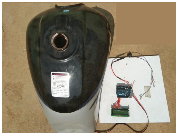
Fig 7 Model Setup for Digital Fuel Level Indicator System for Two Wheeler Vehicles
